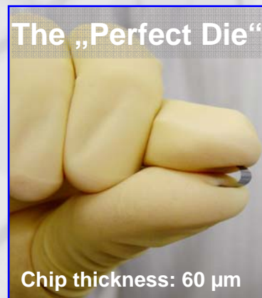
Chip with backside stress relief and with CSH
